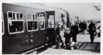
Diesel multiple-units (DMU's) are used on most local rail services (2.25)
